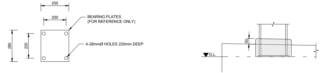
1 BEARING PLATE DETAIL RECESSED INTO SLOPE. FILL RECESS WITH NON SHRINK CEMENTITIOUS GROUT S01 SCALE: 1:10(A1) 1:20(A3)
